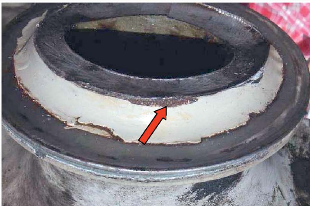
Photo n. 3: presence of uniform corrosion on the external surface, right where the progressive crack initiation.
