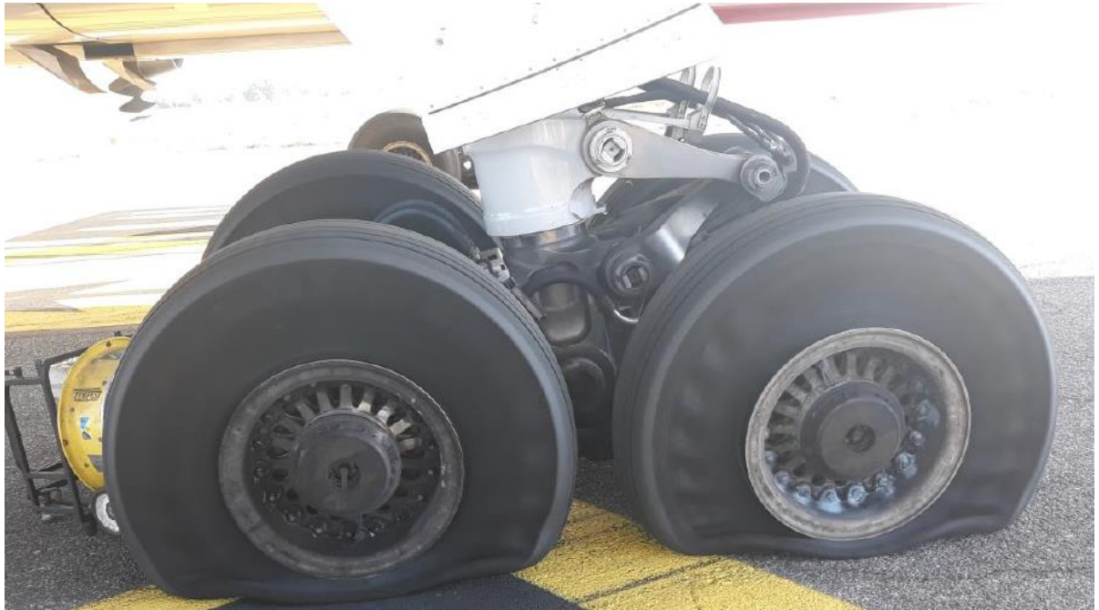
Picture 10: deflated left landing gear tires.
