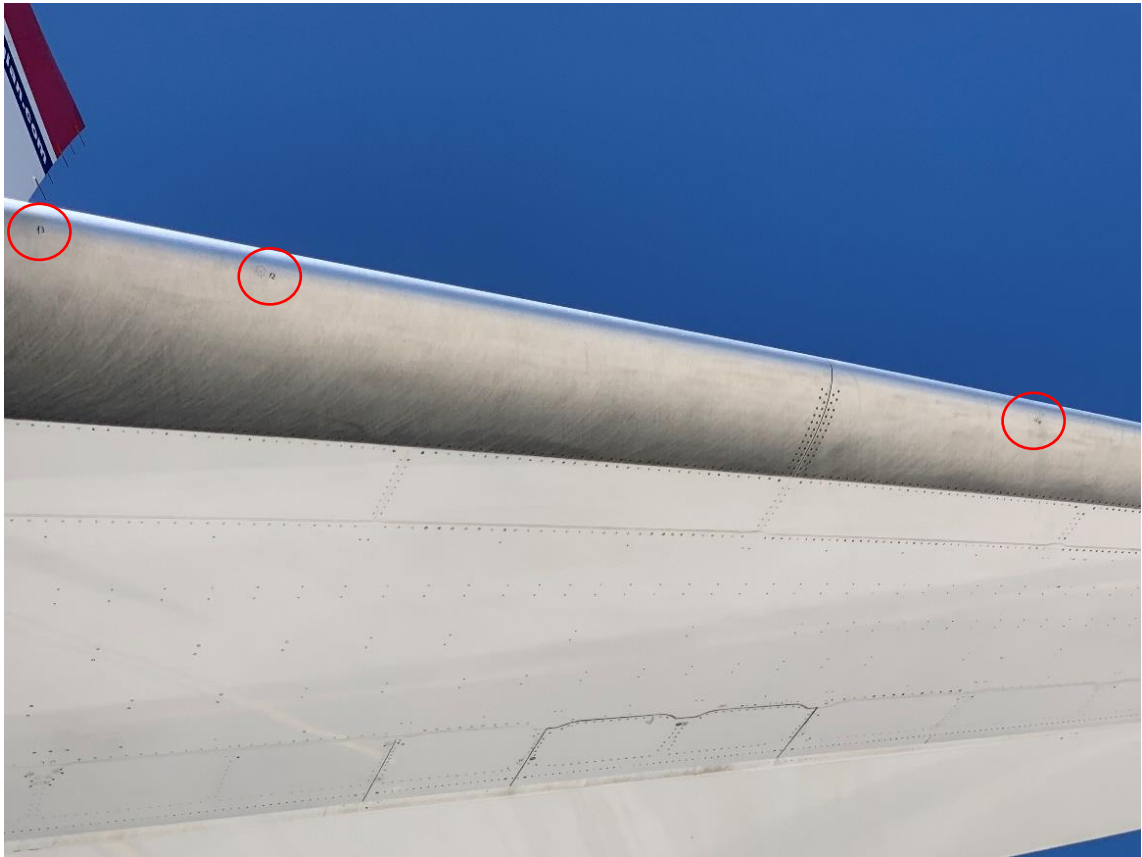
Picture 8: aircraft damage, horizontal stabilizer.
