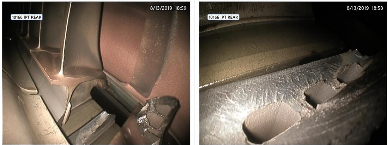
Picture 12: fracture surfaces of the IPT blades found broken.
