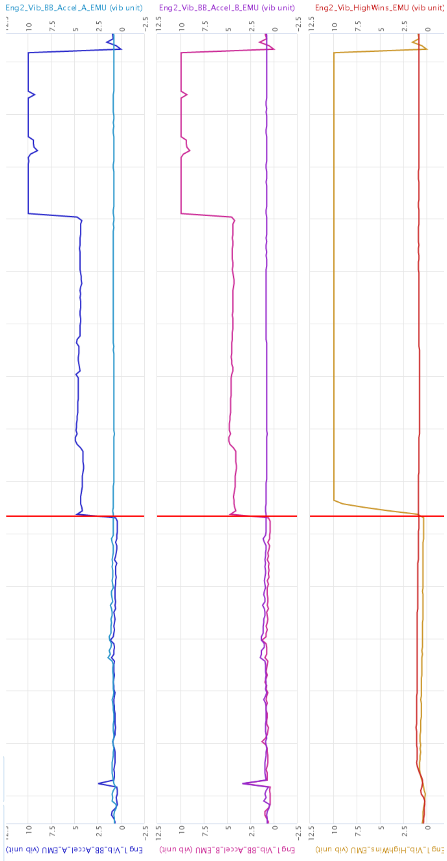
Figure 6: selection of EAFR data, red line 14.46.05 UTC, comparison of ENG1 (left) and ENG2 (right).
