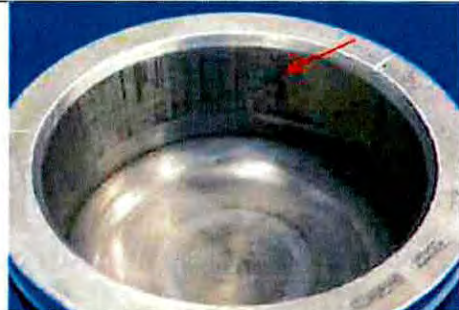
Figure 10: Wear to the piston head inner diameter
