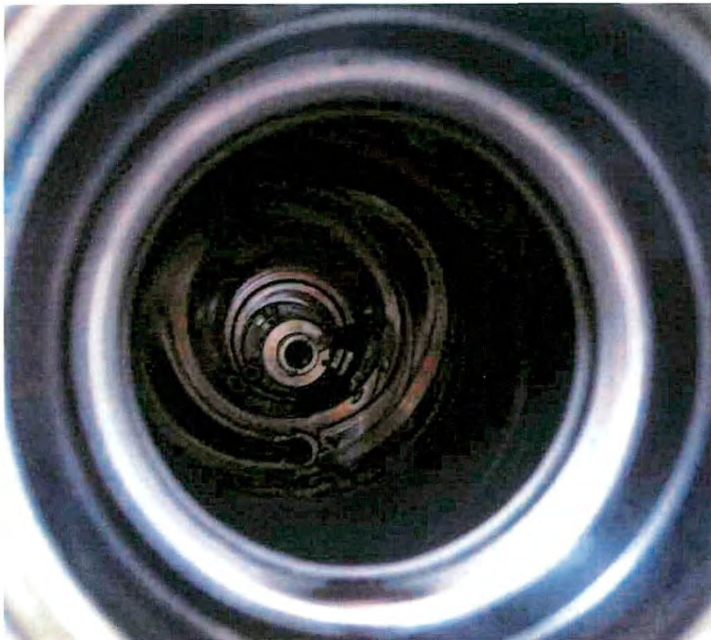
FIGURE 6: TURNING TUBE INNER BORE WITH PISTON, VALVE HOUSING AND RETAINING DOWELS VISIBLE
