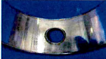
Figure 7: Most wear found on bearing sleeve ID nearest dowel hole 4
