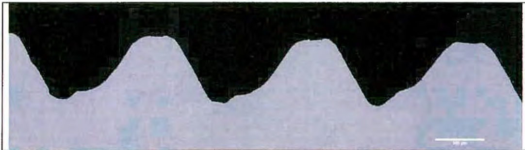
Figure 11: Microsection taken through nut showing incorrect thread form.
