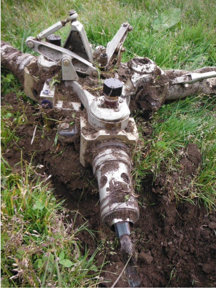
Photo 2: main rotor hub and failed T/T strap.
