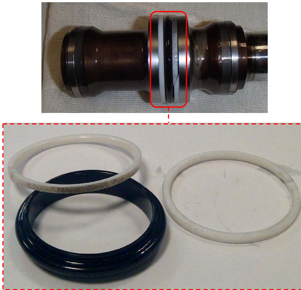
Picture 8: contamination found on LH MLG door actuator.
