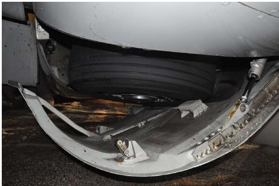
Picture 2: right main landing gear partially open.
