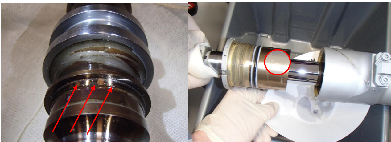
Picture 7: contamination found on LH MLG door actuator.
