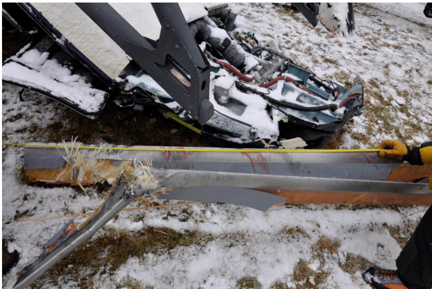
Photo 9: helicopter main rotor blades damages.
