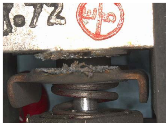
Picture 6: relay return spring
