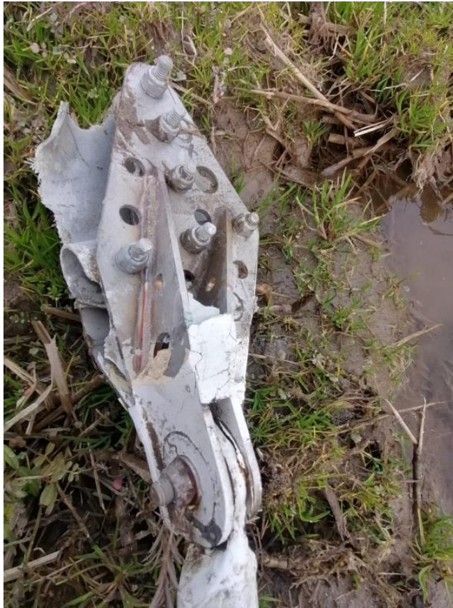
Photo 10: detail of the right wing strut: lower fixing point detached from the fuselage.
