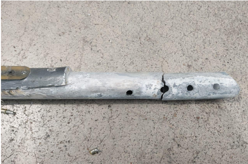
Photo 25: fracture of the aluminium tubular rib at the bolt securing the wing strut fixing plates, found on an Italian Seamax M-22 aircraft after the accident at I-7608.
