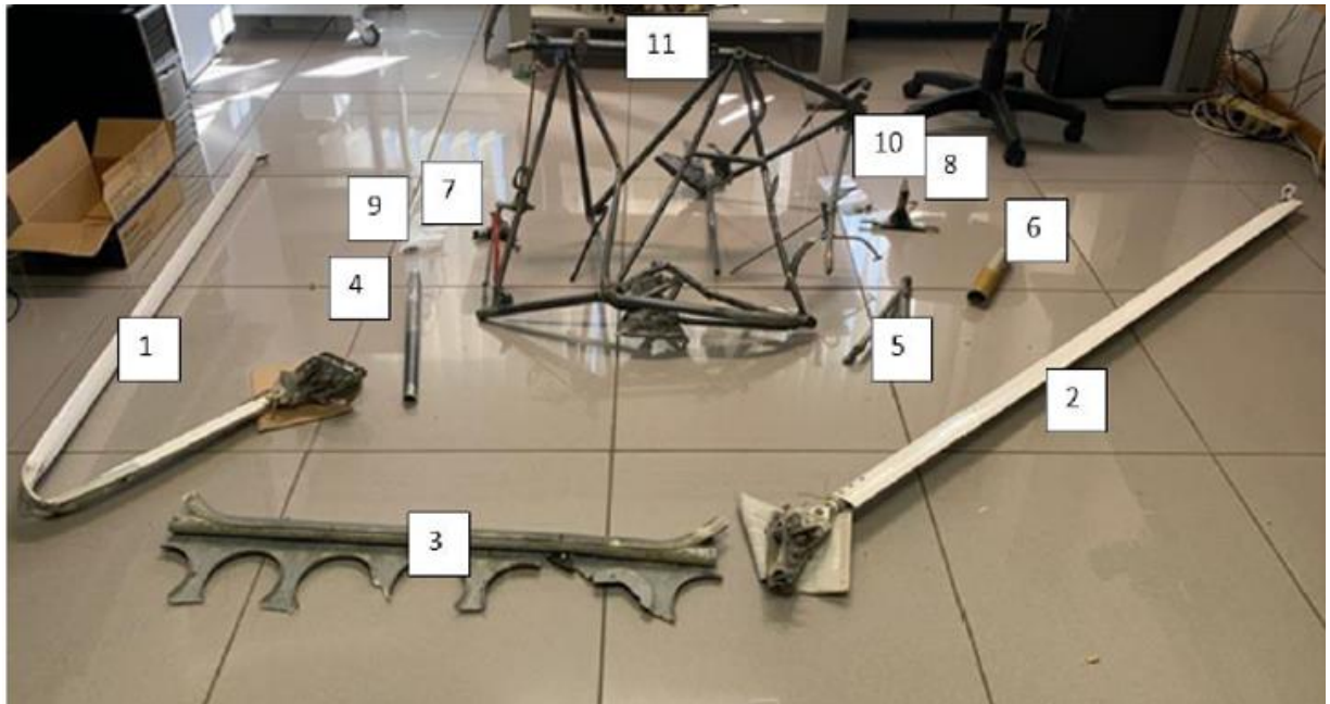
Photo 13: 1. left wing strut; 2. right wing strut ; 3. internal rib wing strut connection; 4. frame rib connection tube; 5. rear right wing connection pin; 6. rear fuselage wing connection; 7. left-side fuselage spar connection mechanism; 8. right-side fuselage spar connection mechanism ( T-shape connection ); 9. wing strut fastening screw left-side wing ; 10. wing strut fastening screw right-side wing; 11. main fuselage steel frame ( cabane ).
