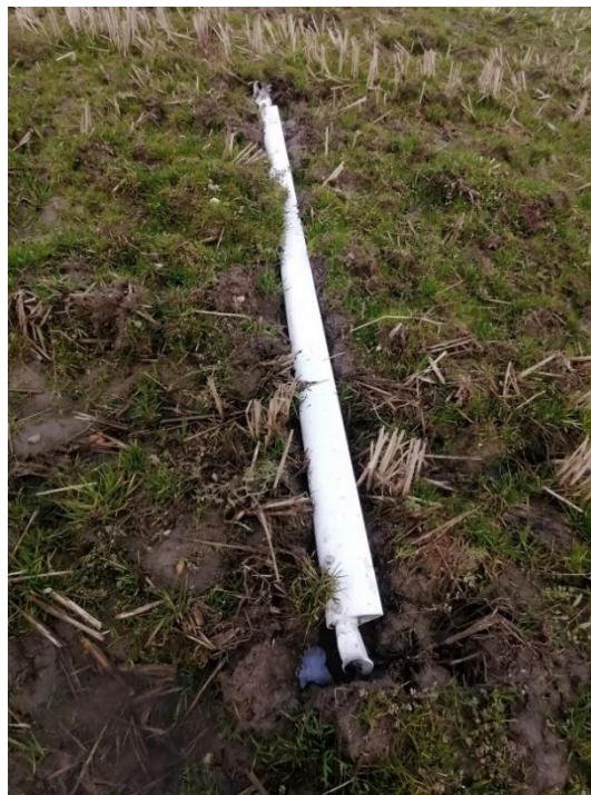
Photo 9: wing strut of the right wing where it was found.
