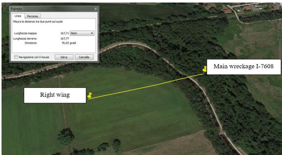
Photo 7: Representation of the positions of the main wreckage and the right wing (on Google Earth support).
