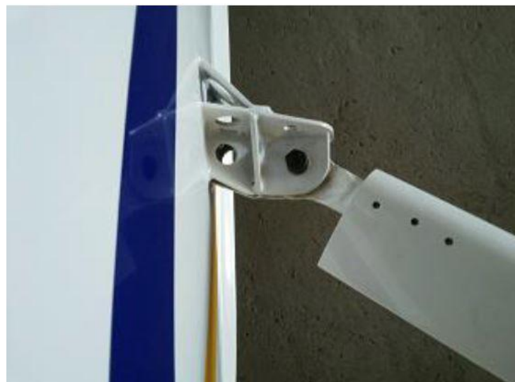
Photo 3: lower fixing point of the wing strut to the fuselage (right wing).
