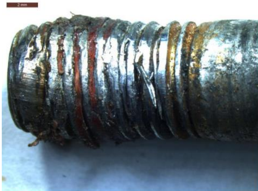
Photo 11: view (optical microscope) of the screw securing the wing strut to the lower part of the right wing.
