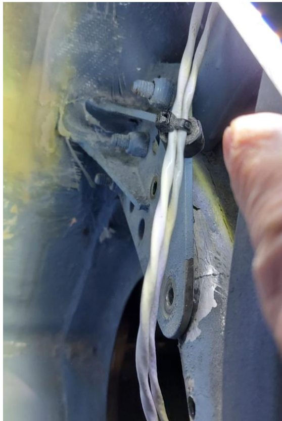
Photo 26: fracture of the aluminium tubular rib at the bolt securing the wing strut fixing plates, found on an Italian Seamax M-22 aircraft after the accident at I-7608.
