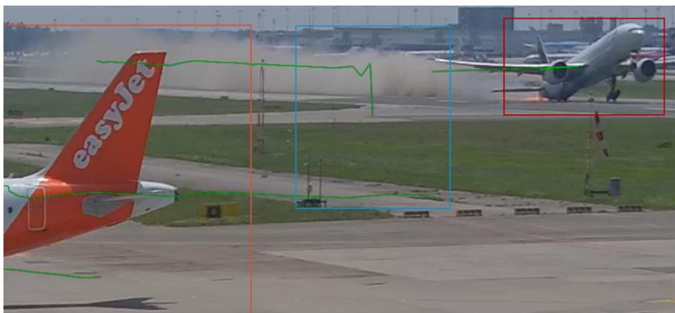
Photo 8: 11.26'49'' main landing gear detached, tail skid still in contact with runway.
