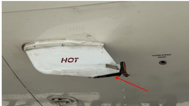
Photo 3: drain mast, indicated by the arrow, detail of the damage.
