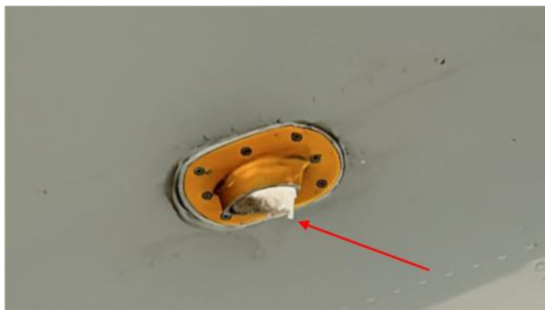
Photo 4: tail strike sensor, indicated by the arrow, detail of the damage.
