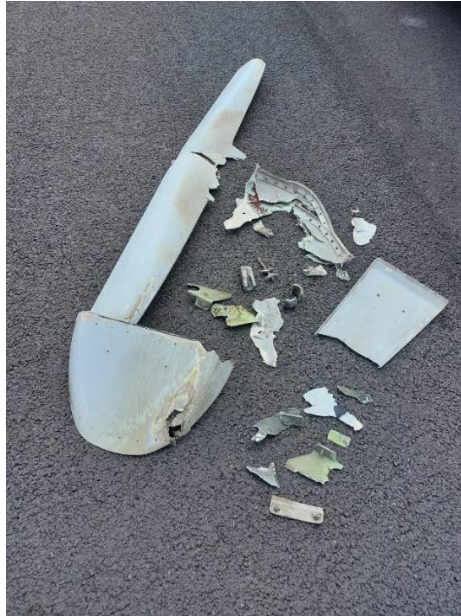
Photo 2: parts of the tail skid assembly found on the runway.
